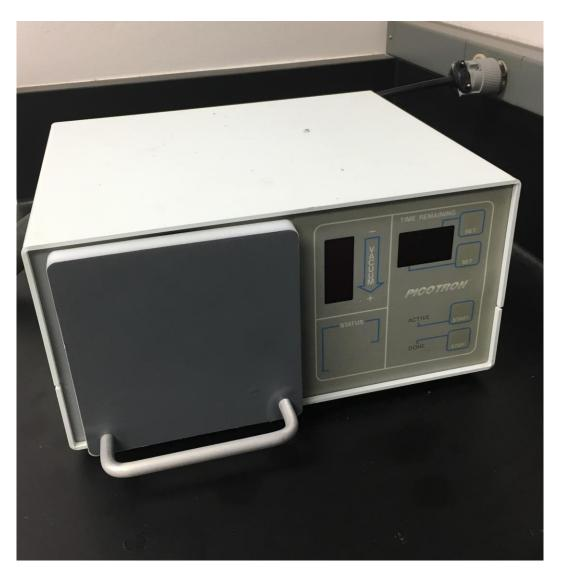
The PicoTron radio frequency glow discharge plasma surface cleaner allows for plasma sputter cleaning of small objects of virtually any dry material. Uses ambient air for plasma generation, other gases are possible with special request and sufficient advance notice.
