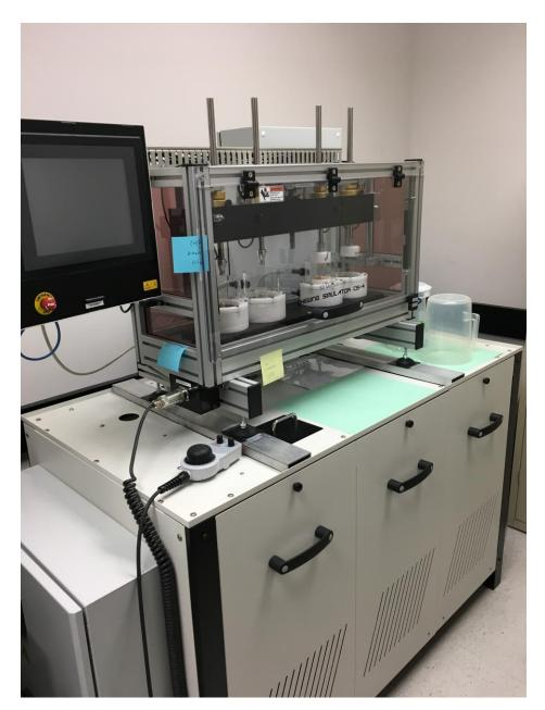
The SD Mechatronik CS-4 Chewing Simulator is an electromechanical dead-weight device that simulates the wear and fatigue caused by chewing. It applies force through either a circular, impact and slide, or impact only pattern. Additionally, it can cycle the temperature of each chamber between 5 and 55 degrees celsius with its built-in water immersion thermocycler. Our machine features 4 chambers that work in sync with each other.
