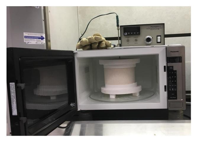
A small desktop programmable microwave sintering oven for use with ceramics. It is capable of reaching temperatures of at least 1400° C and operating at ambient atmospheric pressure. The working volume is a cylinder approximately 5.5 inches in diameter and 2 inches high.
