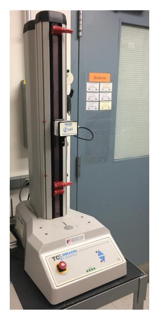
The Dillon TC2i Quantrol is an electro-mechanical universal testing machine with a 500N and a 1000N load cell. We are currently equipped for microtensile and small scale 3 point bending tests. The unit is placed on a vibration dampening table.
