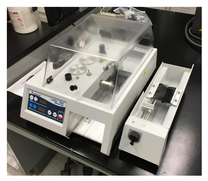
The Isomet 1000 Precision Saw is a gravity fed rotary saw that uses diamond embedded abrasive blades in coolant (usually DI water) to finely section materials. These materials can be almost anything short of diamond. The speed and section width is set digitally. The feed rate is set with a counterbalance and dead weight. A series of fixtures are available for holding materials for cutting.
