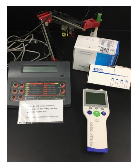
The Mettler Toledo and Hanna digital pH meters allow for general purpose real time testing of the pH of chemical solutions.
