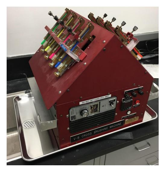
The Sabri V-8 Cross Brushing Machine is designed to simulate the wear from brushing on various surfaces (ex. Composite fillings). The unit has eight chambers and can work with the samples fully submerged.
