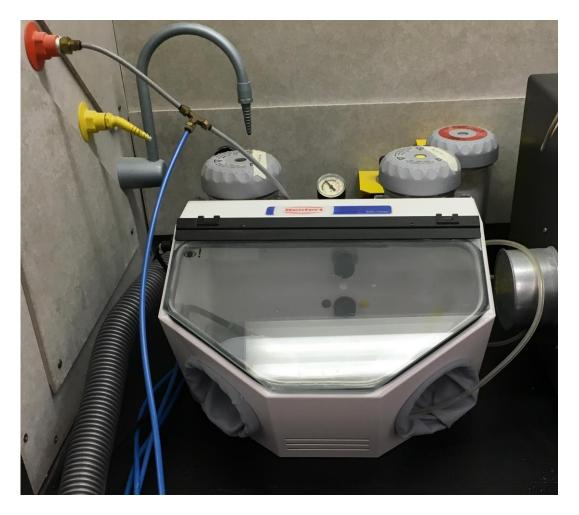
The Renfert Basic Master is a sandblaster for surface modification. It is equipped with alumina (25 - 70 micron), glass beads (70 - 250 micron), and Rocatec blasting media.
