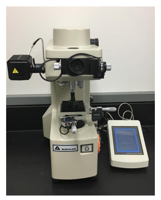
The Buehler Micromet Hardness Tester is a dead-weight micro indentation hardness tester. It has micro Vickers and Knoop indenters with available loads of 10, 25, 50, 100, 200, 300, 500, and 1000gf. It can be used for hardness analysis of thin films, determining depth of hardened layers, estimation of mechanical material values, and more. Curved surfaces can be tested with the micro vickers indenter, and some curvature correction is possible for regularly curved surfaces.
