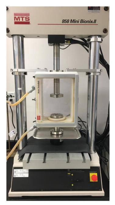
The MTS 858 Mini Bionix 2 is a hydraulic universal testing machine with a 10kN load cell. Its integrated water bath allows for testing at body temperature in wet environments. It is primarily used for cyclic fatigue, tensile, and compressive tests. Currently we have grips for tensile testing and are building a new underwater fixture.
