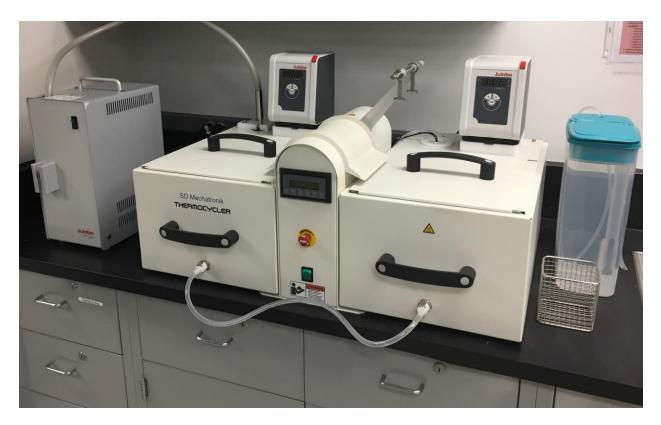
The SD Mechatronik Thermocycler is a device that cycles a basket of samples between two water baths; typically held at 5 and 55 degrees celsius. It simulates the thermal shock of materials (ex. bonded metals) in the mouth during eating and drinking.
