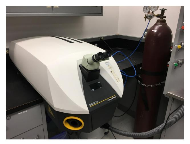
The BEGO Laser T Plus is a laser welder for welding small objects (example: dental crowns, dental bridges, dental retainers). It uses a 1064 nm ND:YAG laser with an argon gas curtain to weld gold alloys, CrCo, Palladium, Titanium, Nickel Titanium, and other commonly available dental metal alloys. It can perform spot and continuous welds.
