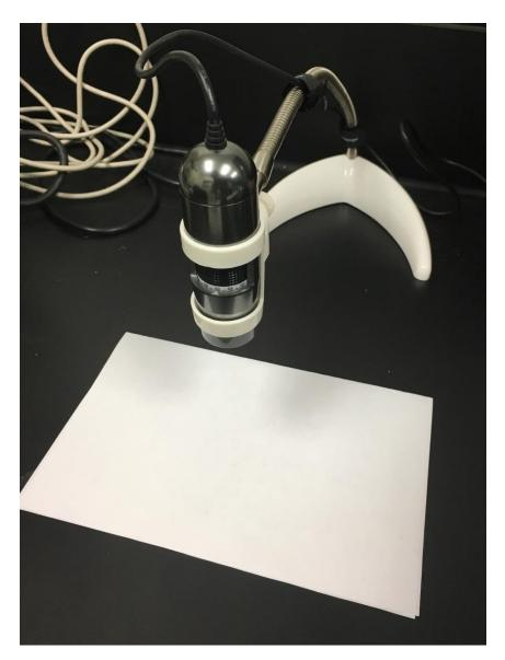
The Dino X Lite digital stereo microscope and its associated measurement software provide a convenient system for easy imaging, measurement, and documentation of samples.
