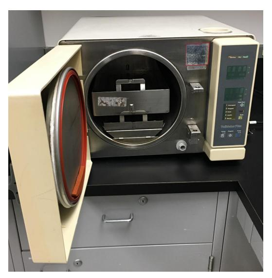
A small desktop steam autoclave for sterilization of small equipment for experiment use. It is capable of sterilizing: unwrapped equipment, wrapped equipment, packs, and liquids. It can also accept limited custom programs.
