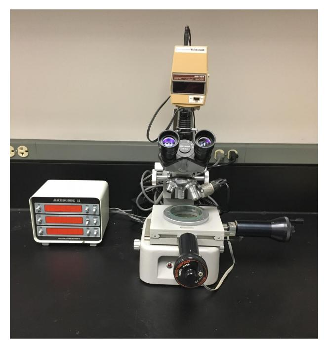
The Unitron Measuring Optical Microscope is used for measuring a variety of samples and features (ex. cracks) with its moving stage and digital readout (accurate to four decimal places). It is capable of measuring the X, Y, and Z axis.
