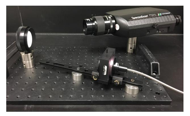
The SpectraScan PR 670 is a spectroradiometer for analyzing visible light spectra. It analyzes the visible color spectra of either an illuminated monitor or a surface under illumination. The device can perform measurements at a distance or close-up; outputting data as a color spectra.
