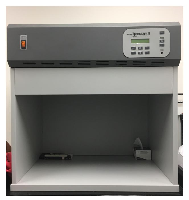
The Spectra Light 3 is a light booth with a series of standardized light sources for replicating various common lighting conditions. The available options include: daylight, cool light, horizon, TL84U30, "A", and UV. Each setting may be used with or without UV. It can also cycle through the lighting conditions.
