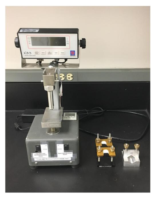
The Ultradent Ultratester is a "micro" shear tester intended for testing samples embedded in PMMA or other resin. To a limited extent, it can be fitted with other fixtures for operations such as flexural testing.
