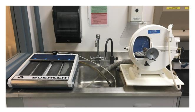
These devices are used for rough and final sample preparation for adhesive shear bond testing and microscopy.
