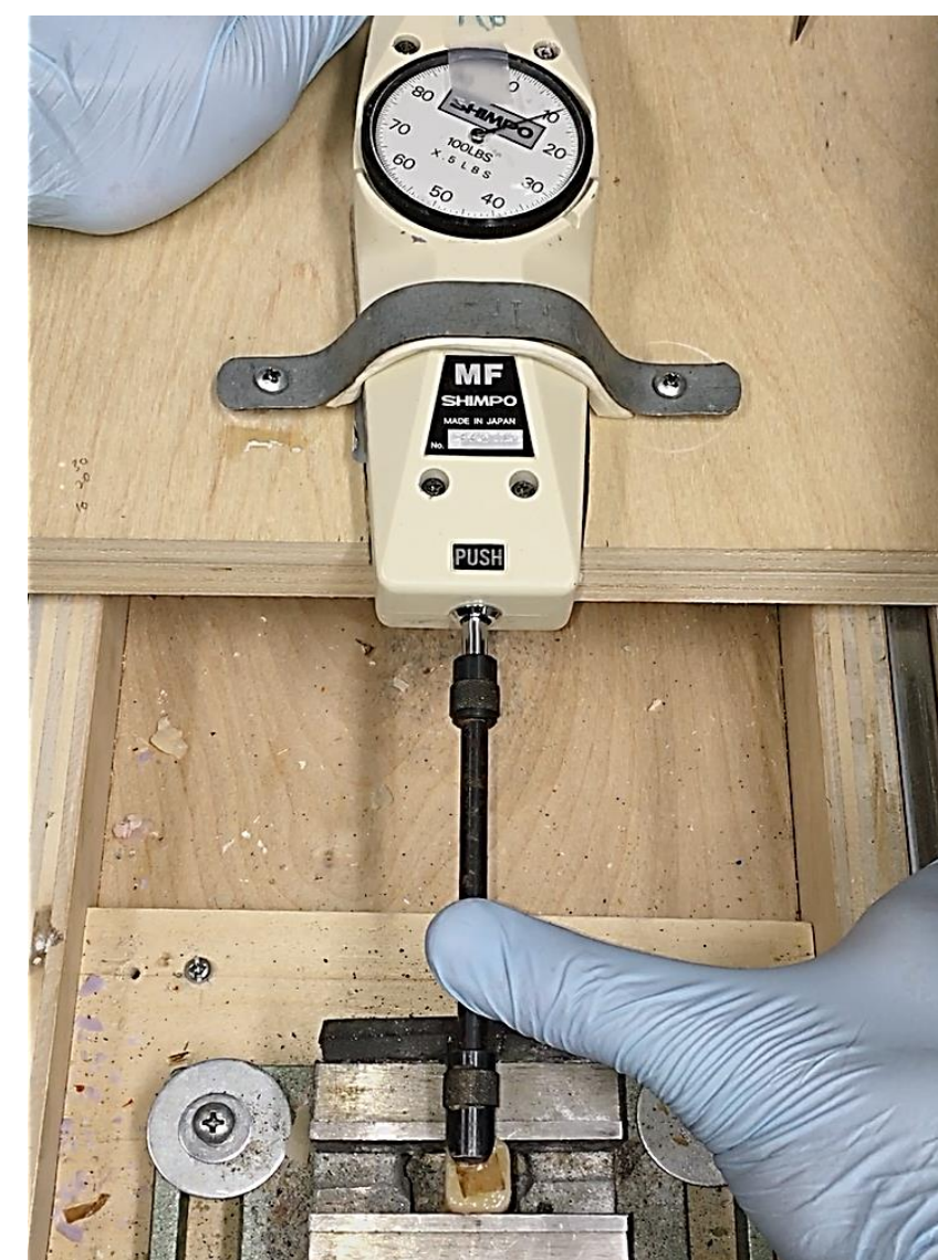
Figure 3. Performing a push-off test using the Shimpo Mechanical Force Gauge
