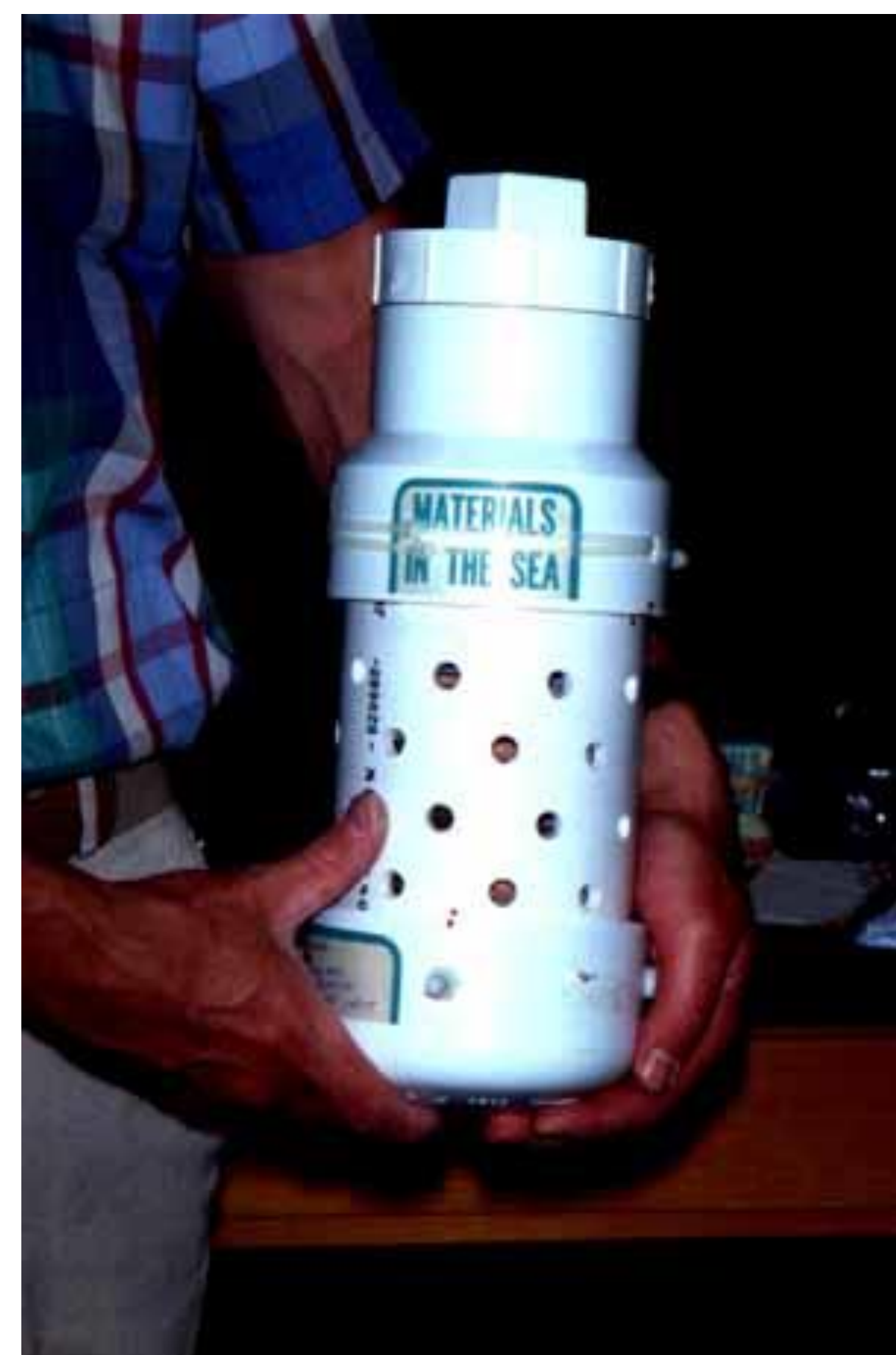
Figure 1: Ballast Organic Biofilm (BOB) sampler
