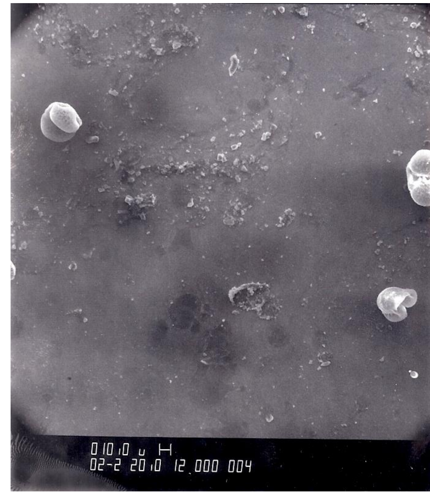
Figure 2: Scanning electron micrograph of typical bacteria-dominated biofilms from ballast tank coupons carried around the world, as found using the Ballast Organic Biofilm sampler.
